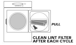
Do not operate the dryer without the grid in place.
